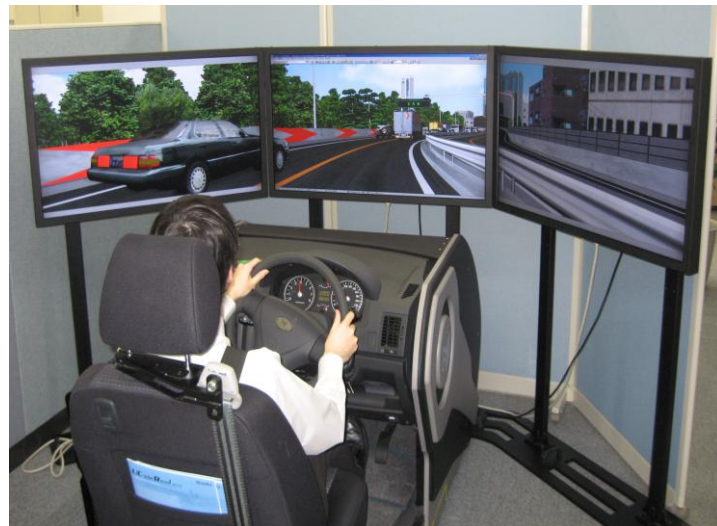
Fig. 5. Full-size 3-panel simulator allows for interaction with the virtual driving environment.
