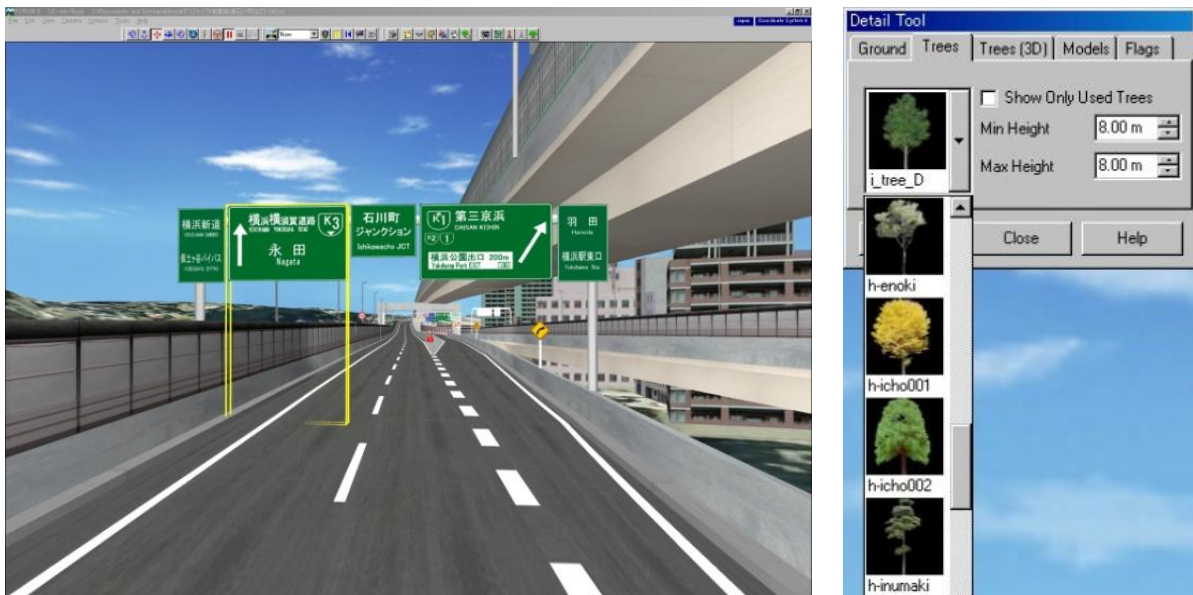
Fig. 4. Sign position editing in 3D interface (left), Detail Tool for adding foliage models (right) (3).
