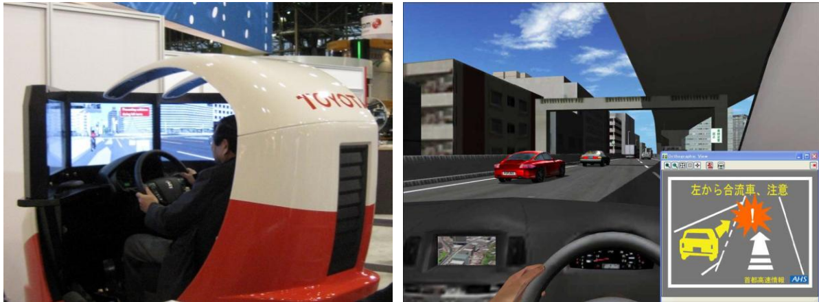
Fig. 9. A motion platform simulator for Toyota's "Integrated Safety Management Concept" system (8) (left), Screenshot of an obstacle warning system in the Smartway 2007 VR Simulation (9) (right).
