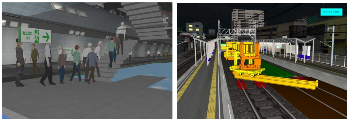
Fig. 10. Animated models observe signage and move from their cars to emergency exits (11) (left), Erection of construction girders for underground construction in train stations (12) (right).
