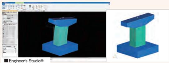
Engineer's Studio®で静的保有水平耐力法の照査
