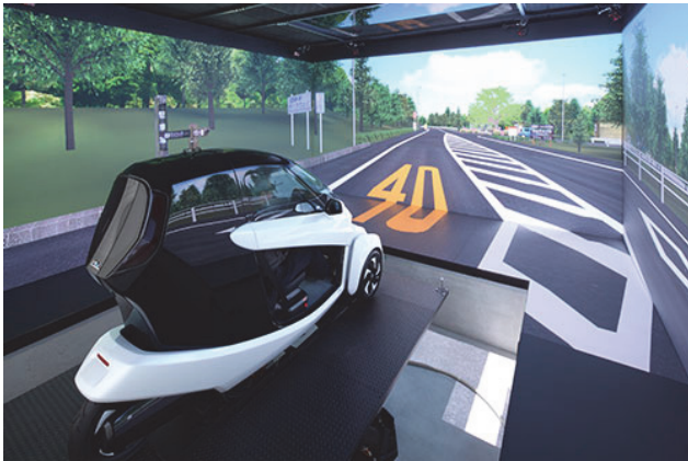
Fig.7 DS with stereoscopic vision of five large screens
