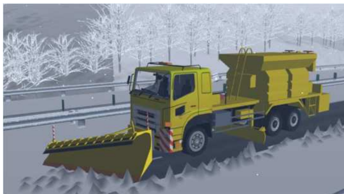
Figure 13 - Snow removal by a truck with one-way snow plow in VR
