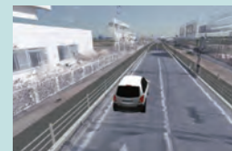
▲ Visualization of collected 3D laser point clouds with UC-win/Road
