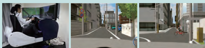
▲ The actual situation of an accident with a bicycle and the surrounding environment are faithfully created with VR to reproduce the situation just before the collision at the timing of running into the road
